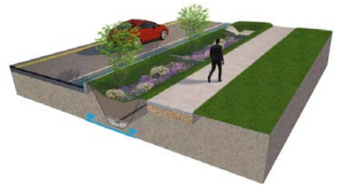
Schematic of a Landscaped Bioretention Swale
